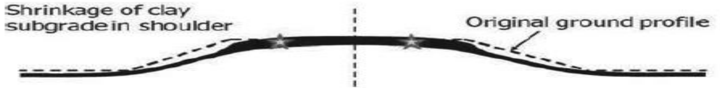
Figure 1. Mechanism of longitudinal crack development on pavement over expansive clays during dry season. (Modified from Zornberg, Gupta & Ferreira, 2010).
